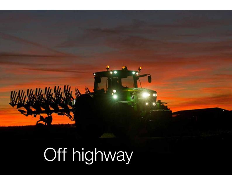
The off-highway segment is a strong growth area. Here the Alfdex solution is applied on diesel engines for tractors, forestry equipment, generators, boats, combine harvesters, military vehicles, locomotives and construction vehicles.
